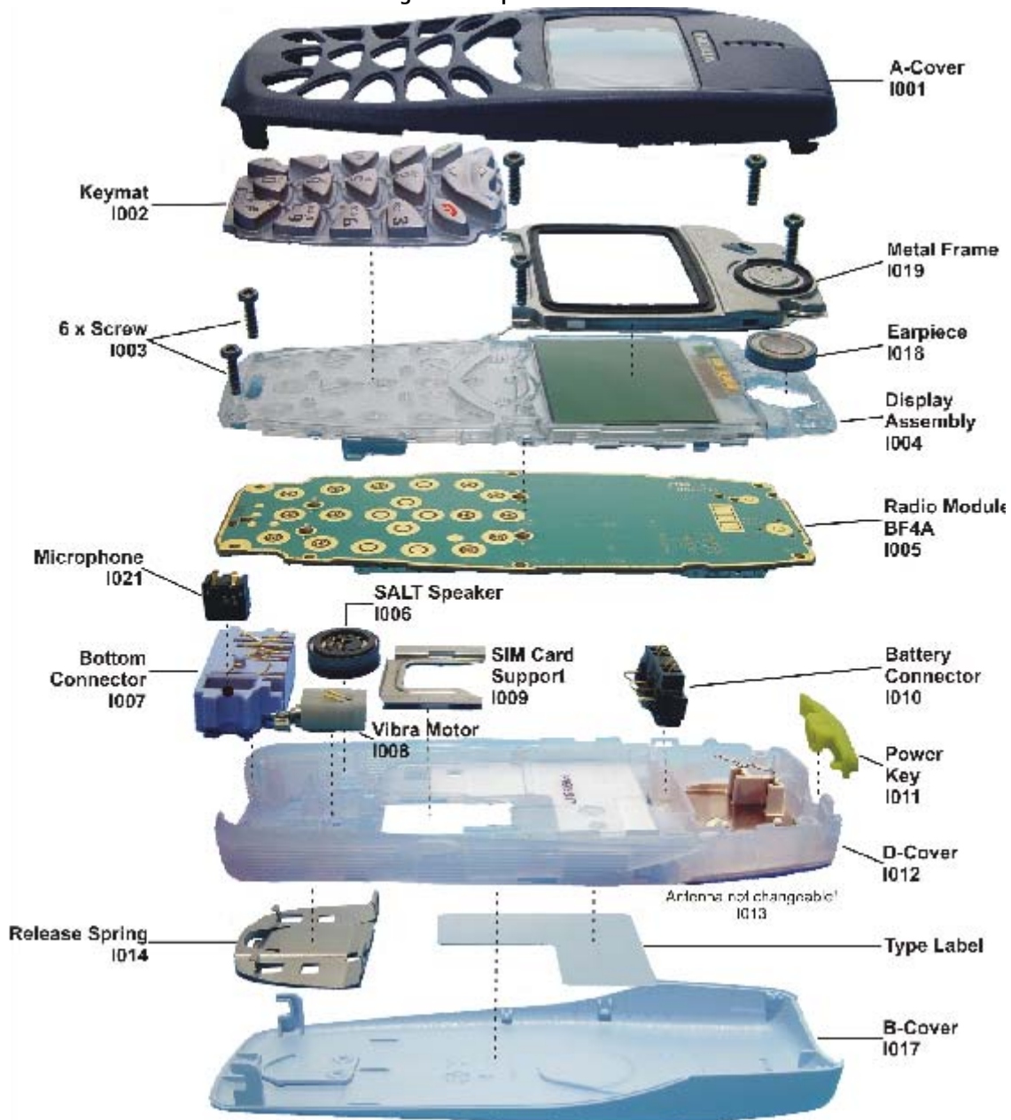
Figure 2: Exploded view of RH-9
